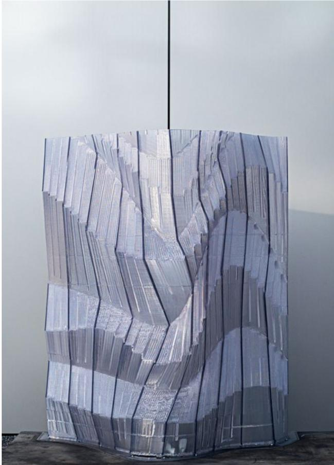
*React/Refract* is a project that explores the intersection of computational design, robotic additive manufacturing and circularity. The prototype uses environmental parameters to create a unique 3D-printed sculpture that combines micro- and macro-patterns to reflect and refract light within a recyclable mono-material. The result is a structure inspired by organic shapes, in which a dynamic and purposeful interplay between light and shadow creates a new aesthetic language.
